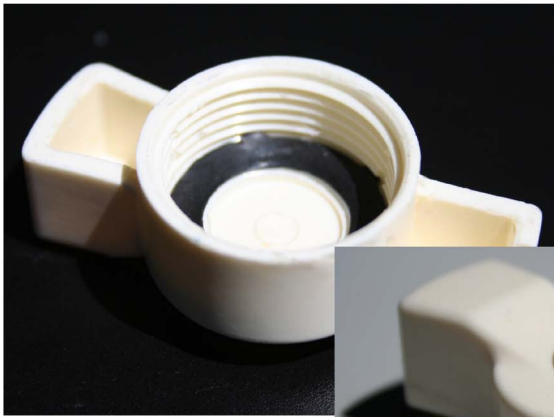
CAST URETHANE CAPS WITH GASKET FOR SEAL TESTING
